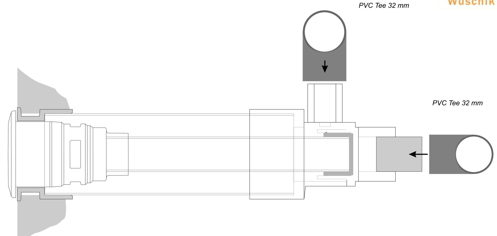
Nozzle insert with 32 mm tube and screw-in adapter bring in.
